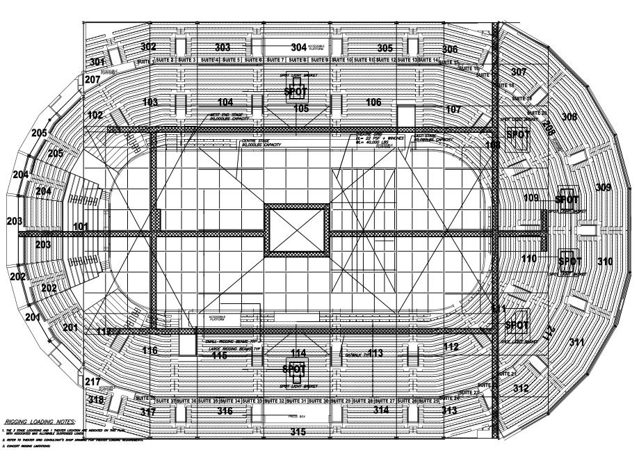
d) THE MAX. RIGGING LOAD ON LARGE RIGGING BEAMS IS 6000 Lbs.
